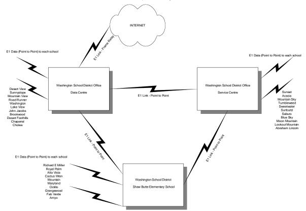
TCP/IP and Novel IPX will be the only networking protocols that will be acceptable to traverse the district WAN. All other protocols will be filtered at the individual school sites using routers. Routers will also be installed at each WAN core location. Access to the "Internet" or any other outside network connections will be provided via the District Office through a frame relay WAN link. For security purposes, no other connections will be permitted.
